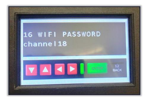
5. Go back and press and hold ENTER. The ^ carat will show up again under O. Up arrow and change to 1 to re-enable Wi-Fi.
